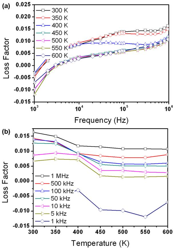
Fig. 3. (a) Frequency dependence of the loss factor after heating at different temperatures. (b) Temperature dependence of the loss factor at different frequencies.
