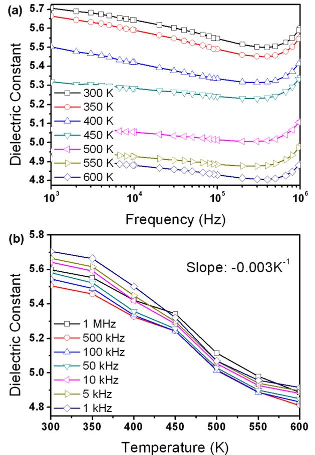
Fig. 2. (a) Frequency dependence of the dielectric constant at different temperatures. (b) Temperature dependence of the dielectric constant at different frequencies and the temperature coefficient of the dielectric constant extracted from the average linear slope.
