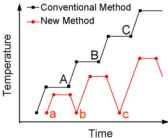
Fig. 4. Comparison of the conventional and the new methods to investigate the temperature dependence. Dielectric properties are measured at points A, B and C in the conventional method and at points a, b and c in the new method.
