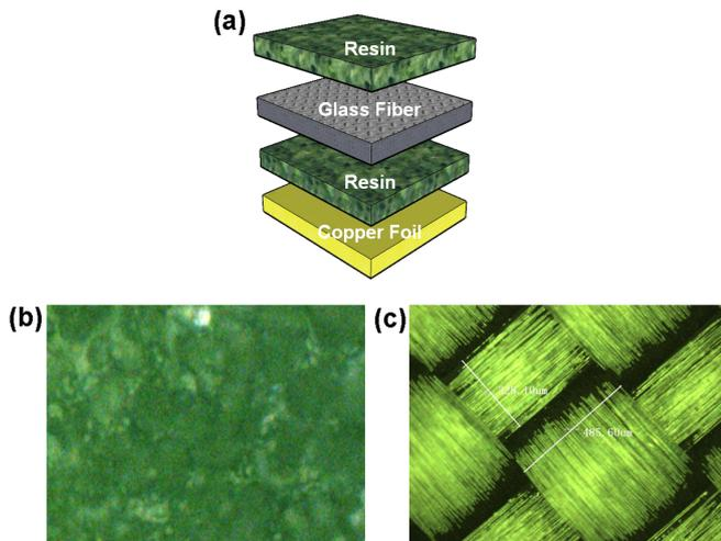
Fig. 1. (a) Separated structure of the single-sided PCB substrate, including resin, glass fiber and copper foil. (b) Resin surface at a magnification of 50. (c) Glass fiber at a magnification of 10.
