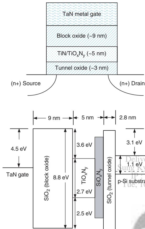
**Fig. 3.** (A) Schematic of the device structure, and (B) energy band diagram at flat band condition of n-MOS transistor memory device with  $\text{TiO}_x\text{N}_y/\text{TiN}$  embedded in  $\text{SiO}_2$ .
