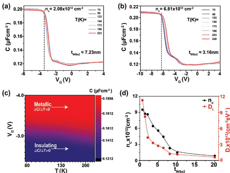
**Figure 2.** Metal-insulator transition driven by traps. a,b) Capacitance-voltage curves of  $\approx 7.23$  nm and 3.16 nm thick  $\text{WSe}_2$  devices measured at various temperature points, respectively, where the dotted black vertical line indicates the MIT point. c) Color-code plots of the 7.23 nm thick  $\text{WSe}_2$  device. d) Critical carrier density ( $n_c$ ) and corresponding trap density ( $D_t$ ) versus thickness of  $\text{WSe}_2$  flake ( $t_{\text{WSe}_2}$ ).
